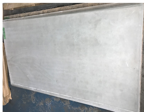
Fig. 5. Appearance of panel after pyrolysis. (Panel with intact cover glass).
