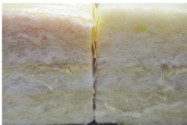
Fig. 13. Appearance of the prototype. (Left: prototype derived from solar panel glass; Right: product made from conventional materials).
