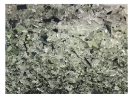
Recovered Materials After Sorting (Undersize Fraction)
