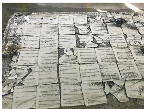
Fig. 3. Appearance of panel after pyrolysis. (Overall view of the panel after heat treatment).
