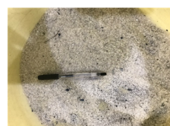
Recovered Materials After Sorting (Light Fraction)
