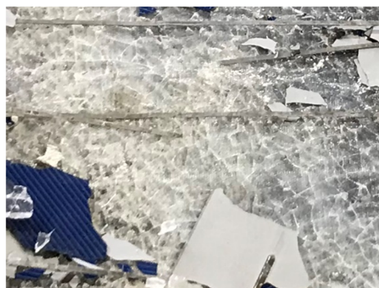
Fig. 4. Appearance of panel after pyrolysis. (Close-up view of the glass section after heat treatment).
