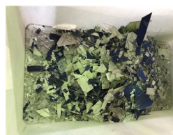
Recovered Materials After Sorting (Oversize Fraction)
