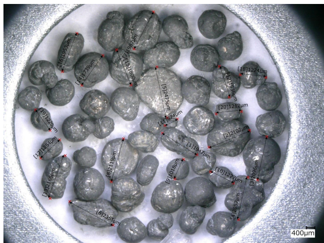
Fig. 6. Solder balls (0.6~2.5 mm) recovered from panel after heat treatment.
