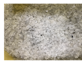
Recovered Materials After Sorting (Heavy Fraction)
