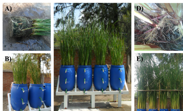
Fig. 4. A) System at the start of operations; B) system with 5 weeks of maturation; C) system with 4 months of maturation; and E) complete growth of the rhizosphere throughout the forced flotation container.
