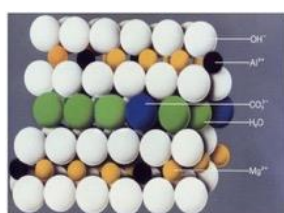
Fig. 1. Schematic diagram of HT (Courtesy of Kyowa Chemical Industry Co., Ltd.).
