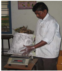
Figure 2. Image of weighing for estimation of physical composition of MSW Of MCE
