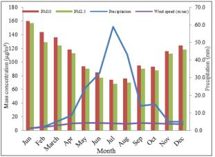
Fig. 7. Monthly variations of  $PM_{2.5}$  and  $PM_{10}$  mass concentration with monthly total precipitation.
