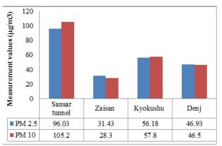
Fig. 4. Hourly average concentration of particulates PM2.5 and PM10.
