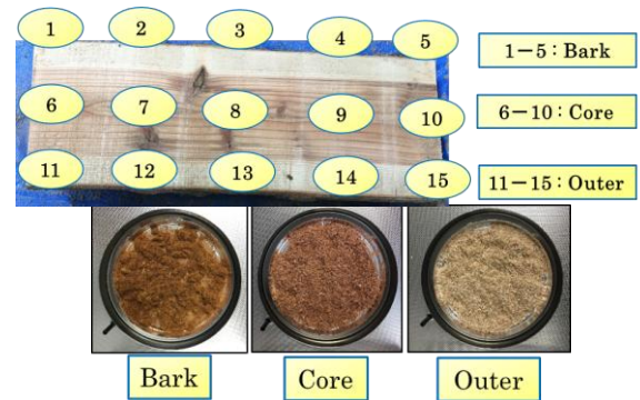
Fig. 3. Sampling points for moisture measurements.
