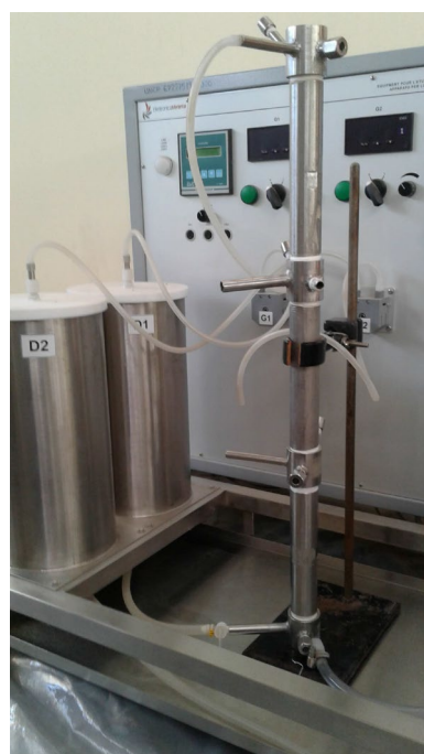
Fig. 3. Stainless-steel fixed-bed reactor used for continuous methylene blue degradation.
