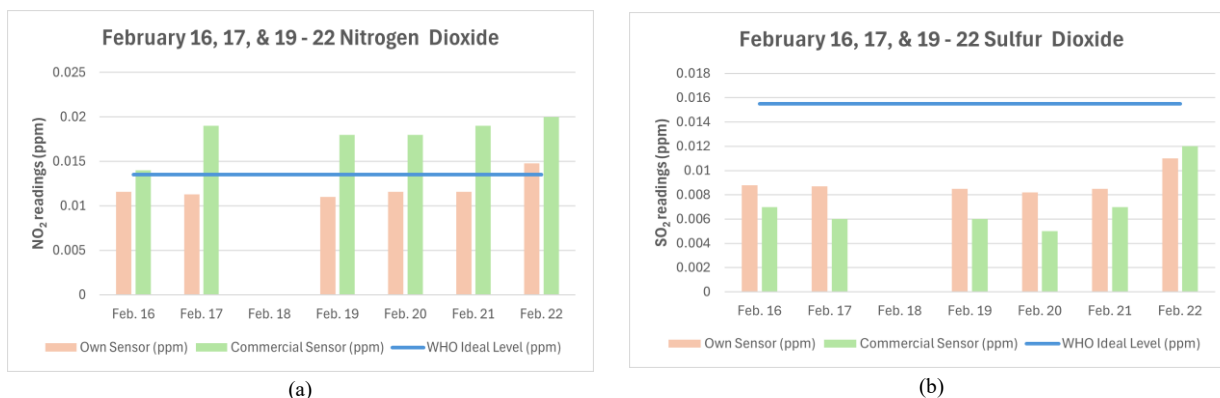
Fig. 5. Sensor comparison against WHO guidelines. Bar graphs comparing (a) NO 2 , and (b) SO 2 readings from the NSOx sensor and a commercial sensor across February dates, with WHO ideal levels indicated. The visualization supports performance benchmarking and compliance assessment.
