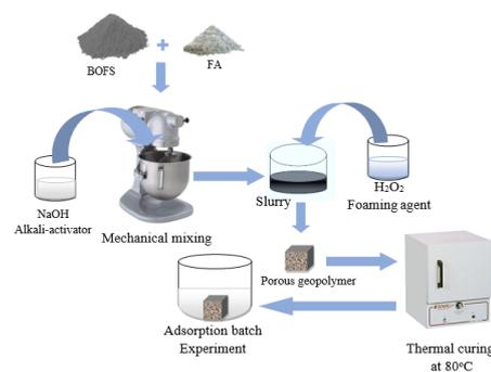
Fig. 2. Schematic diagram of geopolymer synthesis and batch experiment for the removal of metals.
