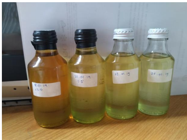
Fig. 8. The re-use of reclaimed oil transformer.
