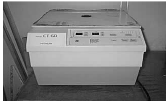
Fig. 3a: Centrifuge dewatering model [4].
