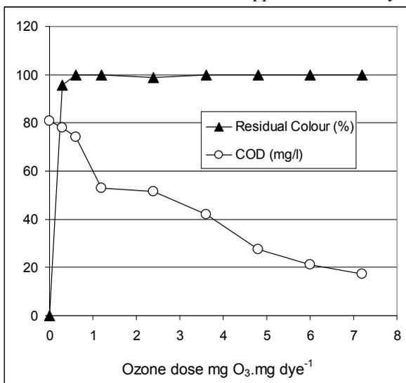
Figure 2. Colour removal efficiency and COD concentration of Reactive Red 120 solution at various ozone doses.
