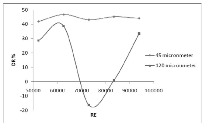
Fig. 7. Relationship between Reynolds number and percentage of drag reduction with different iron particle size for concentration 500ppm at power setting 1200W.
