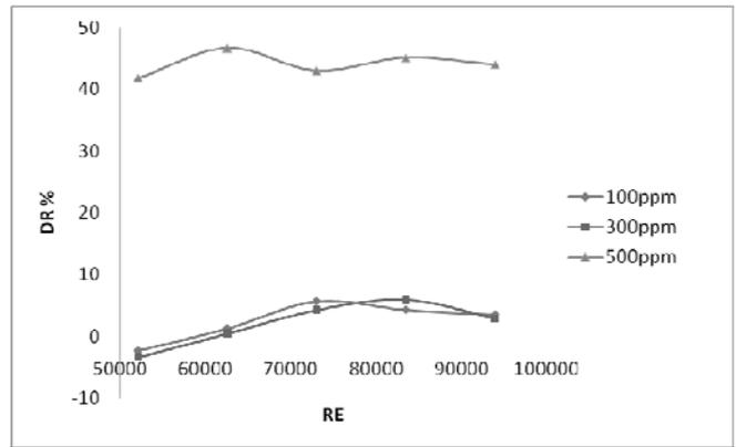
Fig. 5. Relationship between Reynolds number and percentage of drag reduction with different iron particle concentration for size 45µm at power setting 1200W.
