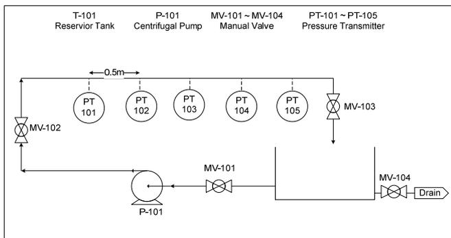
Fig. 1. Fluid friction pilot plant
