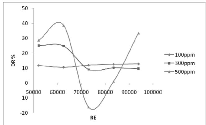
Fig. 6. Relationship between Reynolds number and percentage of drag reduction with different iron particle concentration for size 120µm at power setting 1200W.
