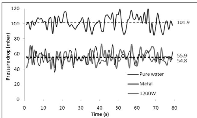
Fig. 4. Behavior of the pressure drop influenced by the magnetic field applied for iron particle 45µm of concentration 500ppm at Re= 83448
