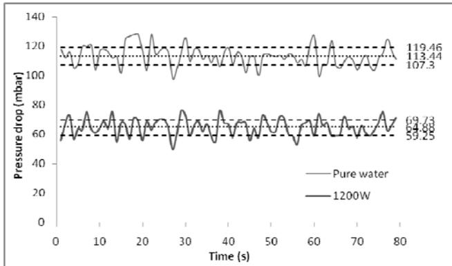
Fig. 3. Behavior of the pressure drop influenced by the magnetic field applied for iron particle 45µm of concentration 500ppm at Re=93879 (compared with pure water)
