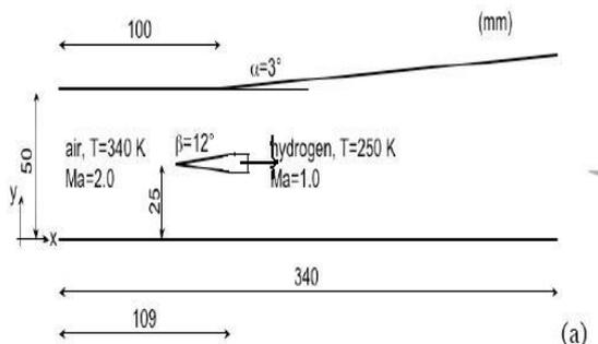
Fig.1 Physical model of Strut based combustor
